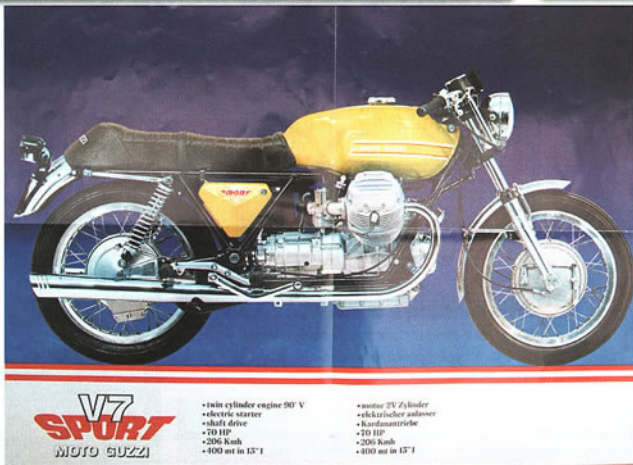
► 1972 The V7 Sport had Lafranconi or Silentium shark-gill silencers, swan neck bars and a triangular lockable toolbox. Pure class
